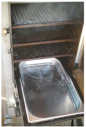
Important note: contrary to the so-called water smokers, the role of the water and water pan is not primary in the BBQ PIT BOX® Cabiner Smokers. Due to their construction these smokers are stable enough without a water pan and there is no need for extra moisturizing in the Cooking Chamber. It has a secondary, minor effect on heat flow, but even with this, the primary function of the Water Pan is to collect juice and grease from the meat.
