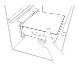
• There is a **Drain Plug** in the V-shaped bottom sheet of the Cooking Chamber. In case we remove it, the water from the high-pressure cleaner drains through the pipe to the **Outer Drain Pan**.
