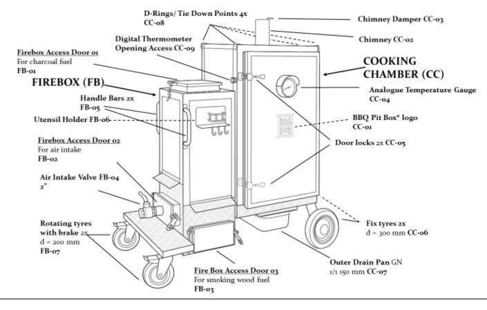
\* The image above is based on Model GF-S.
